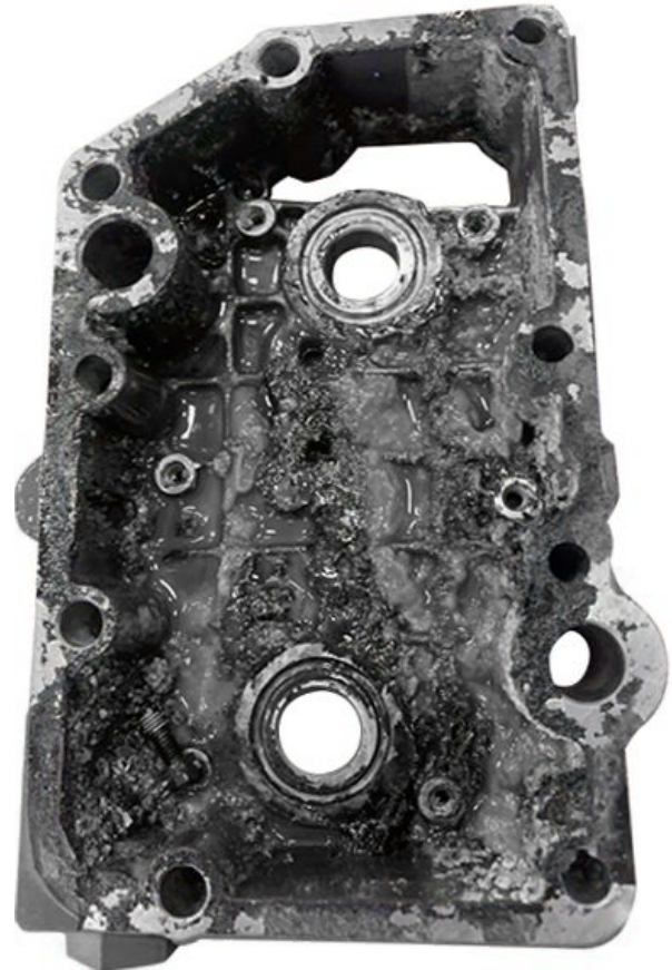
Effects of Prolong Storage of Coolant — More Than One Year
