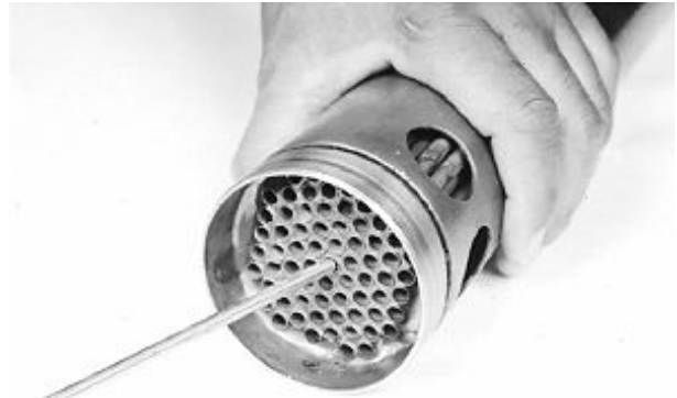
Clean Heat Exchanger
