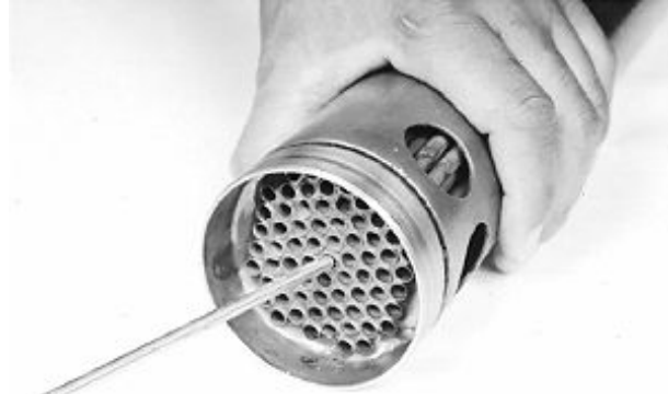
Clean Heat Exchanger
