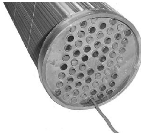
Clean Aftercooler Core
