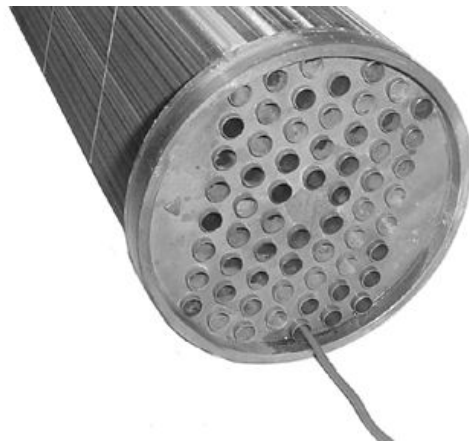
Clean Aftercooler Core
