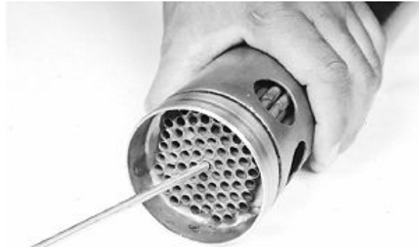
Clean Heat Exchanger
