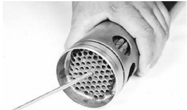
Clean Heat Exchanger
