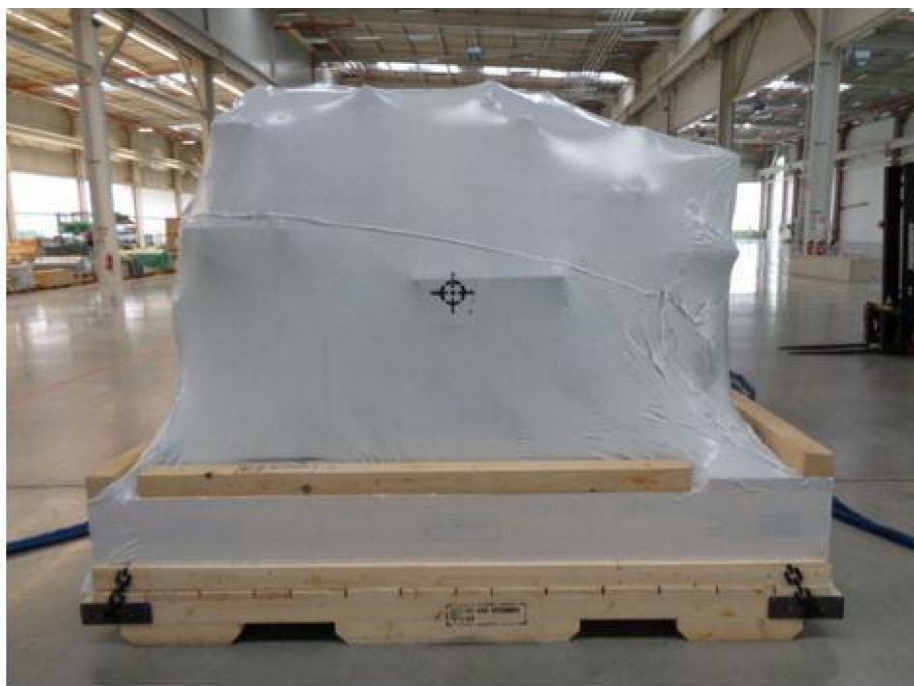
Fig. 41: Example of waterproof packaging
