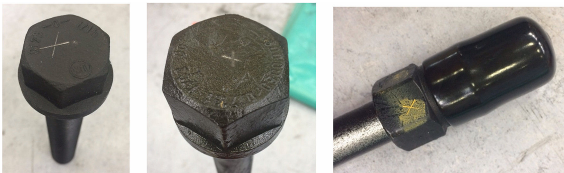
Fig. 106: Examples of markings on screws and HP pipe nut
