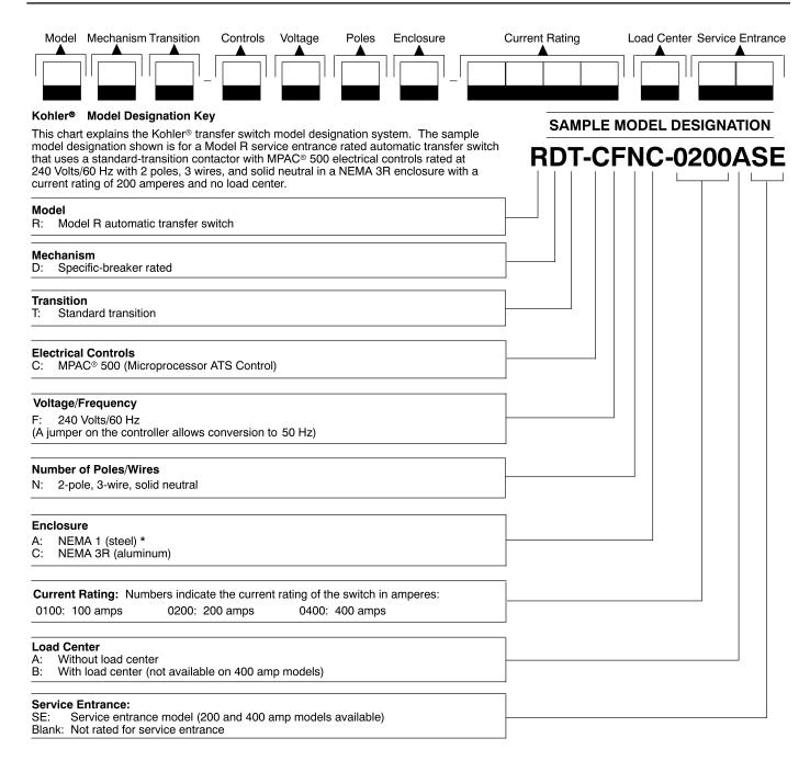
\* NEMA 1 only: 100 and 200 amp models without load centers can be recess-mounted between wall studs. Optional wall-mount bezel available.
