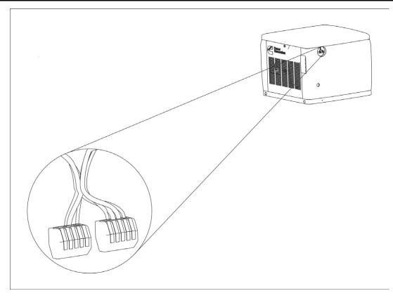
FIGURE 16. CUSTOMER AC CONNECTIONS
