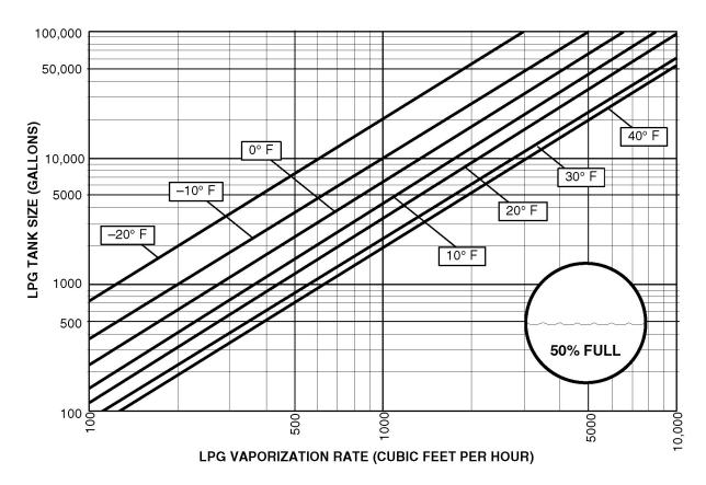
FIGURE 37. MINIMUM LPG TANK SIZE (50% FULL) REQUIRED TO MAINTAIN 5 PSIG AT SPECIFIC WITHDRAWAL RATE AND MINIMUM EXPECTED WINTER TEMPERATURE
