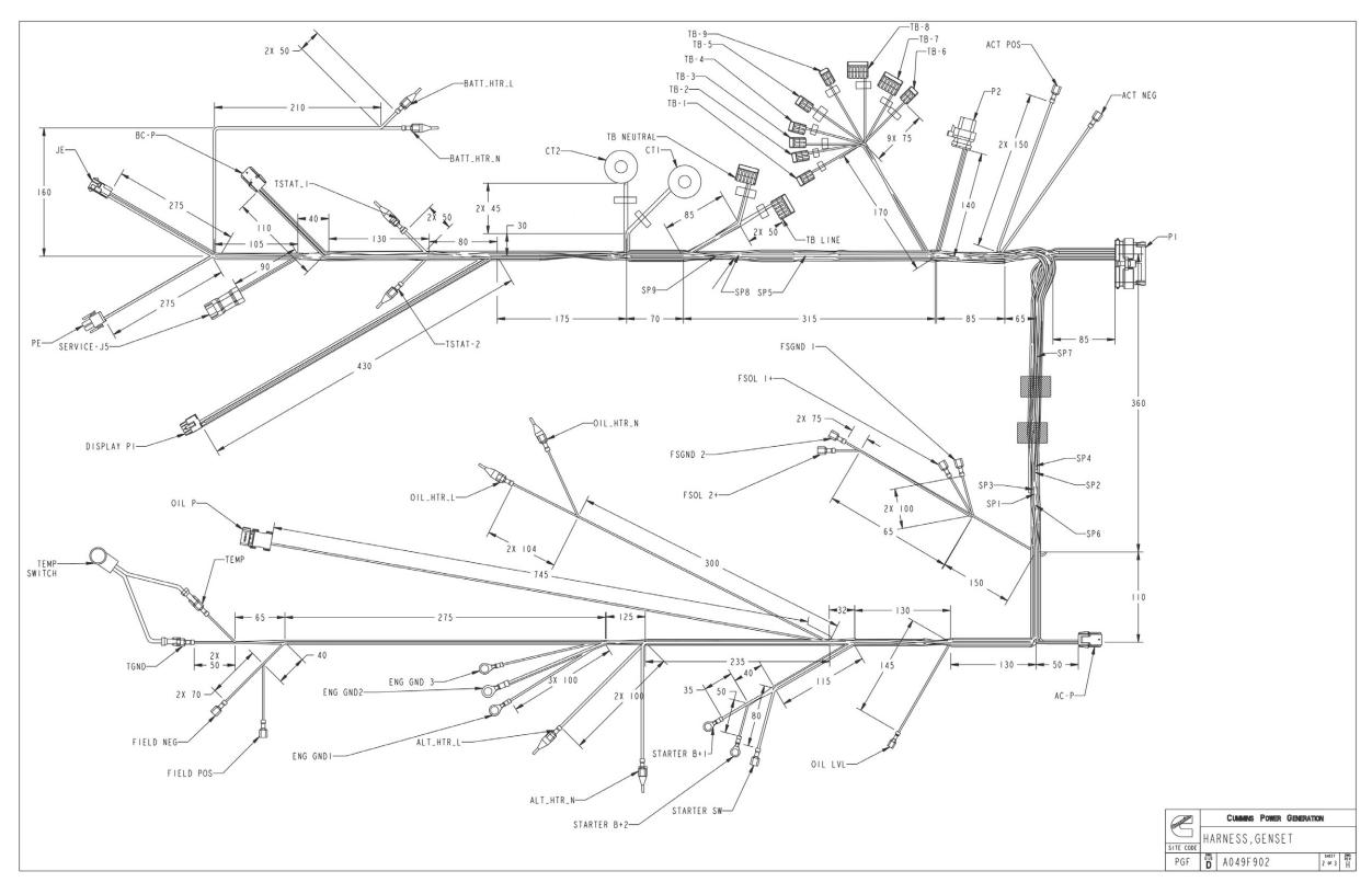
FIGURE 49. HARNESS, GENERATOR SET ELECTRICAL (SHEET 2 OF 3)
