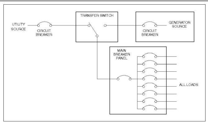
FIGURE 4. TRANSFER SWITCH CONNECTIONS FOR FULL COVERAGE LOAD
