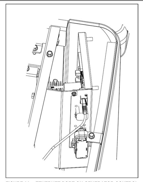
FIGURE 36. ETHERNET PORT ON GENERATOR CONTROL
