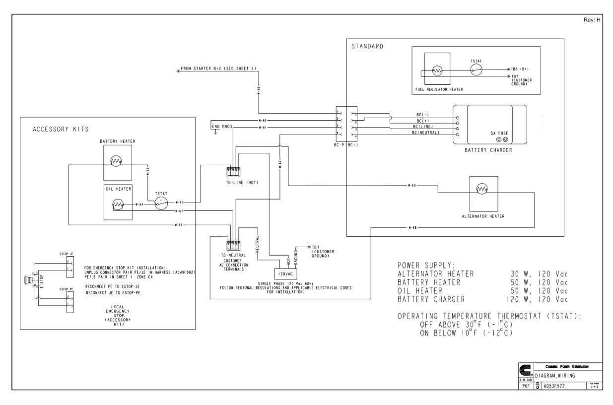
FIGURE 43. WIRING DIAGRAM (SHEET 2 OF 6)
