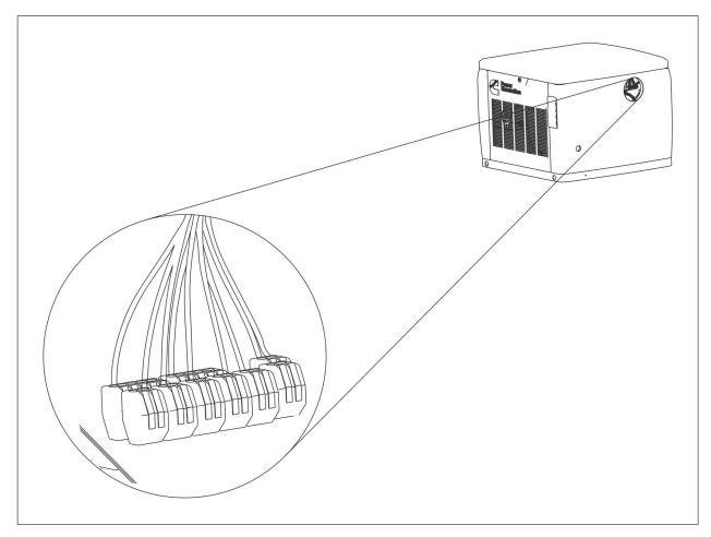
FIGURE 17. LOCATION OF CONNECTION POINTS FOR ATS DC CONTROL WIRES
