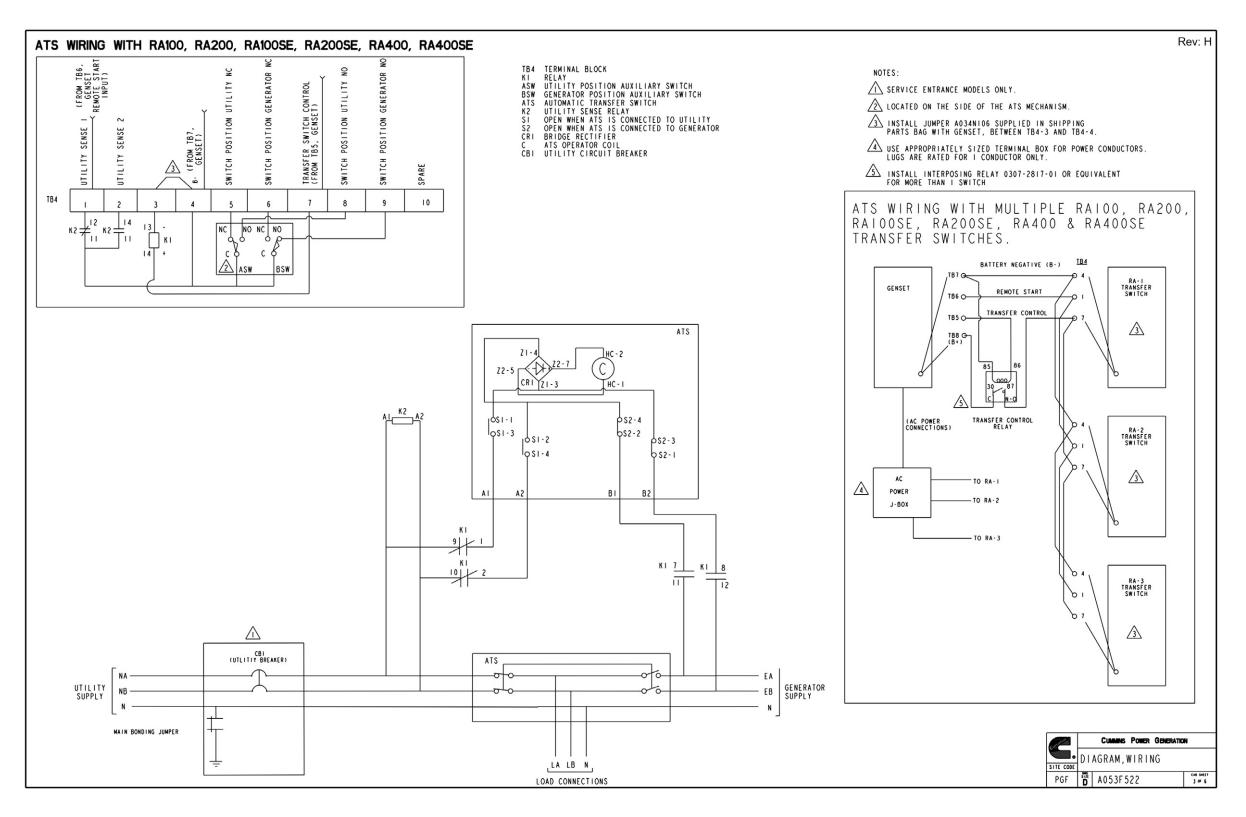
FIGURE 44. WIRING DIAGRAM (SHEET 3 OF 6)
