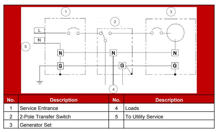
FIGURE 18. TYPICAL SYSTEM GROUNDING ONE-LINE DIAGRAM (SEPARATE SERVICE ENTRANCE AND 2-POLE TRANSFER SWITCH)
