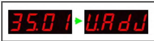
Step 3: Select the phase you wish to re-calibrate by pressing the OFF key.
