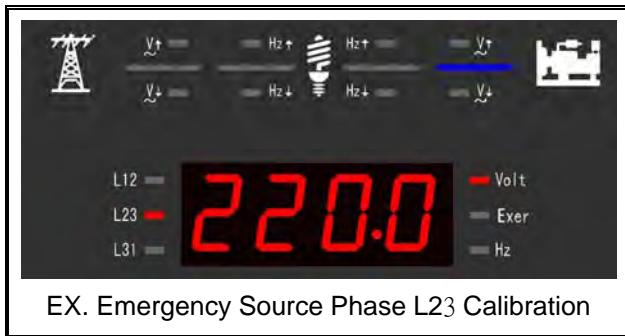
Step 4: Using a good calibrated voltmeter as your reference recalibrate the ATS-22 voltage readings.
