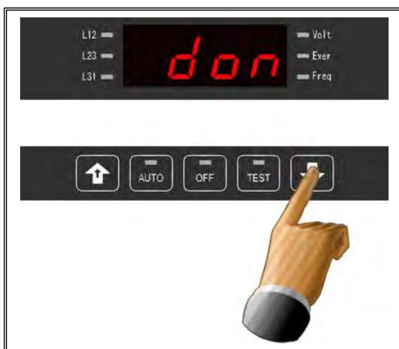
Step 8: After recalibrating all five-touch buttons. The screen displays “End” for 2 seconds and exits the Touch Buttons Sensitivity Adjustment setup.
