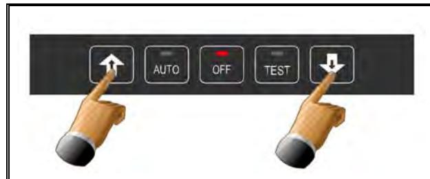
Step 6: Press the "OFF" button to move to the next phase or until the word "End" appears on the screen. To exit hold the "OFF" key at any time for 4 sec.
