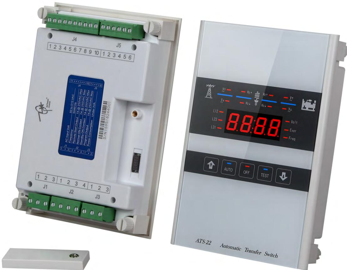
A complete Automatic-transfer-switch PLC controller. It works with most ATS and incorporates all power relays and connections together with the software for each type of ATS. It also has a slot to accommodate a USB, RS485 or Ethernet communications module. Easy to install, easy to program.
