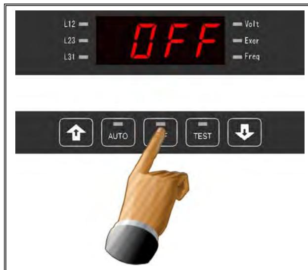
Step 6: When “tEST” appear on the screen, touch the
