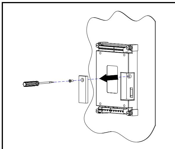
Step 2: Plug in tighten the screw on the KCU-XX module to the ATS-22 PCB.
