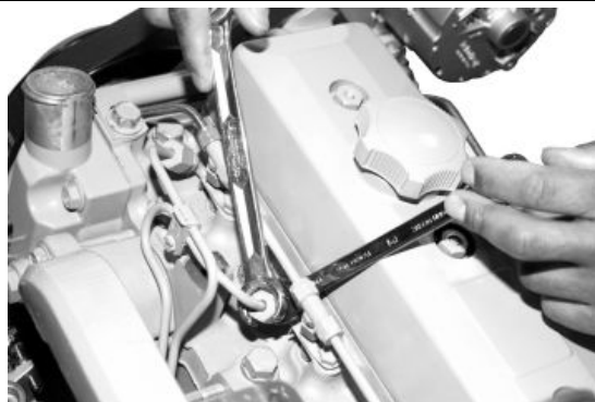
Fuel Line Connection
