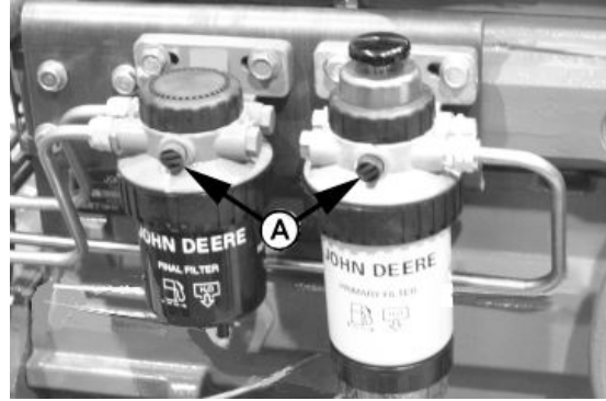
Air Bleed Vent Screws (Final Filter at Left, Primary Filter with Separator Bowl at Right)
